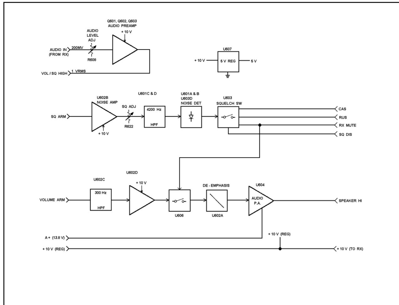
Figure 2 - Audio Board Block Diagram
